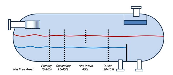
Fig.1: Baffle Applications & Typical Specification
